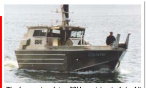
The featured craft is a 32' bowpicker built by All American Marine. Twin 273 jets, directly driven by 315hp Cummins 6BTA diesel engines, provide thrust for a lightship speed of 42 mph. As the jet impellers are rated to constantly absorb the full power output of the engines regardless of boat speed, the engines cannot be overloaded when travelling under load at slower speeds.
