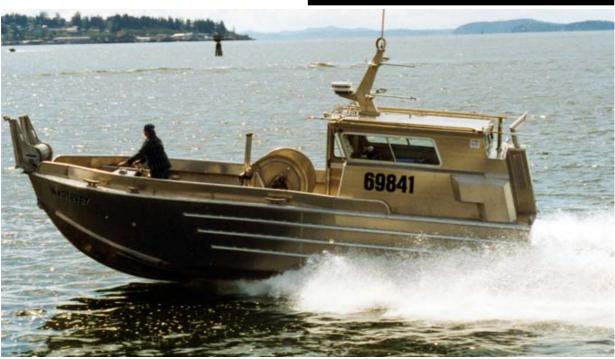
The salmon fishing fleet in Cordova AK has an extensive fleet of older bowpickers, with many powered by Hamilton 1031 waterjets and 460 c.i.d. Ford gasolene engines. New replacement craft entering service in this busy fishery are being fitted with Hamilton Jet 273 pumps and diesel engines.
