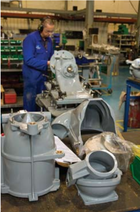
Above: The 10,000th HJ212 waterjet in final assembly at the HamiltonJet Factory
